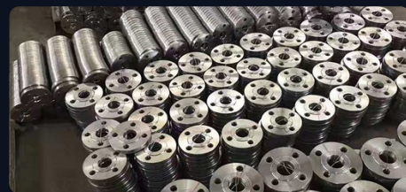
Machined flanges awaiting inspection
