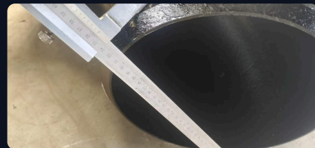
Dimensional check with vernier caliper
